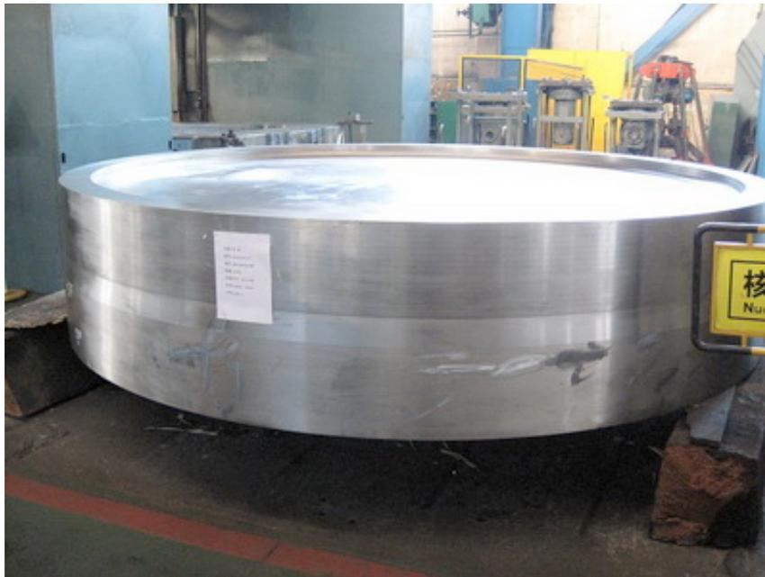
Similar, but smaller, Tubesheet image – prior to drilling for tube insertion
